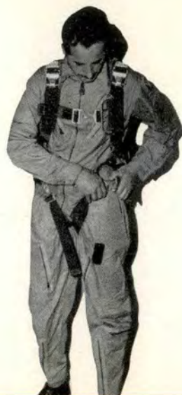
The Class III harness is the latest, with pre-set aneroid chute opening.
