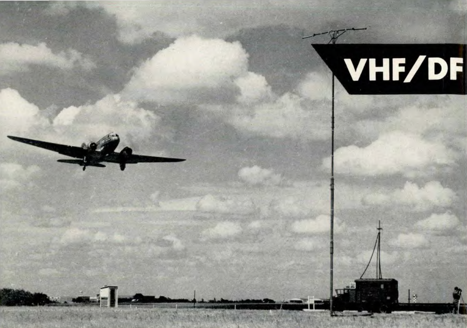
AACS plane from Tinker AFB flies over a VHF/DF unit to check its accuracy. Such in-flight inspections are made every 90 days.
